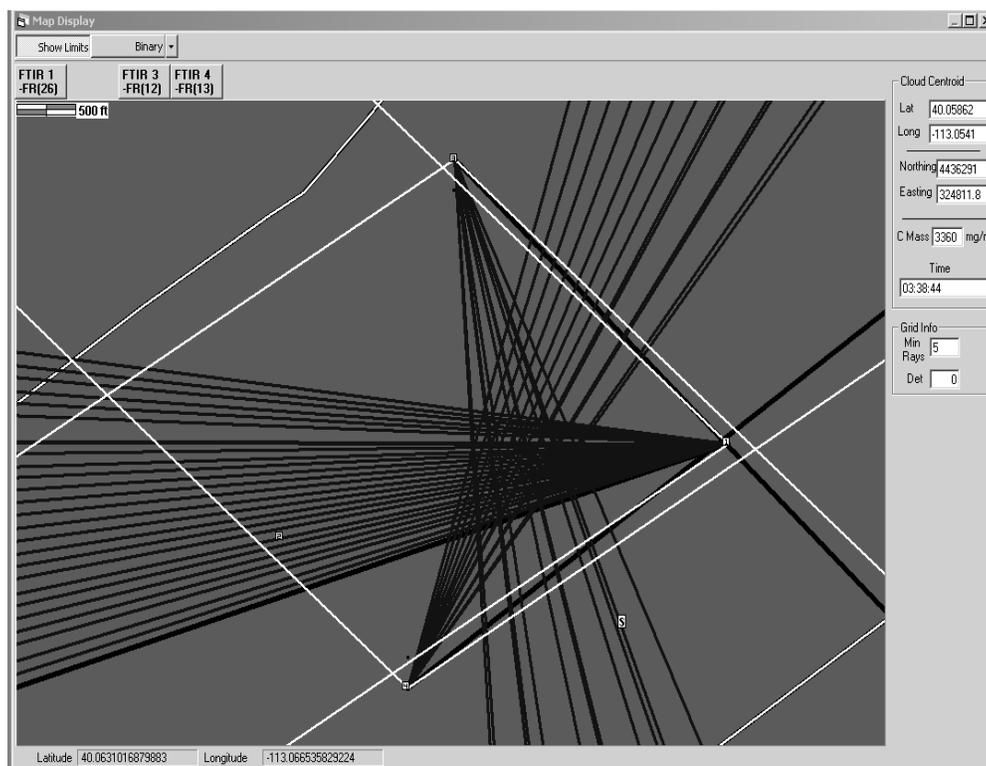
Fig. 4 – A typical set of CL measurement vectors from 3 FTIRBoxes after scanning the truth box.
