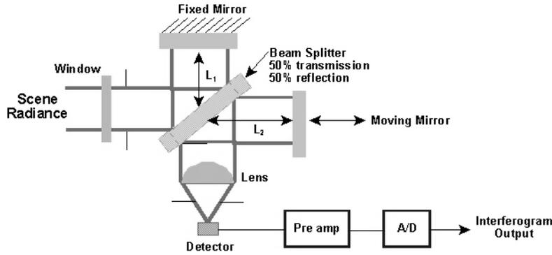
Fig. 1 – Michelson FTIR sensor schematic.
