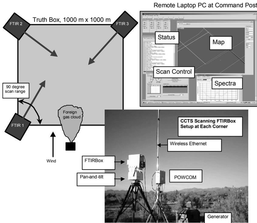
Fig. 3 – CCTS diagram including equipment setup and command post software display.
