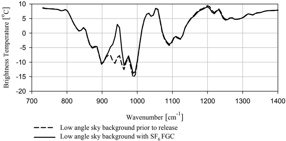
Fig. 5 – SF<sub>6</sub> FGC release brightness temperature spectra.
