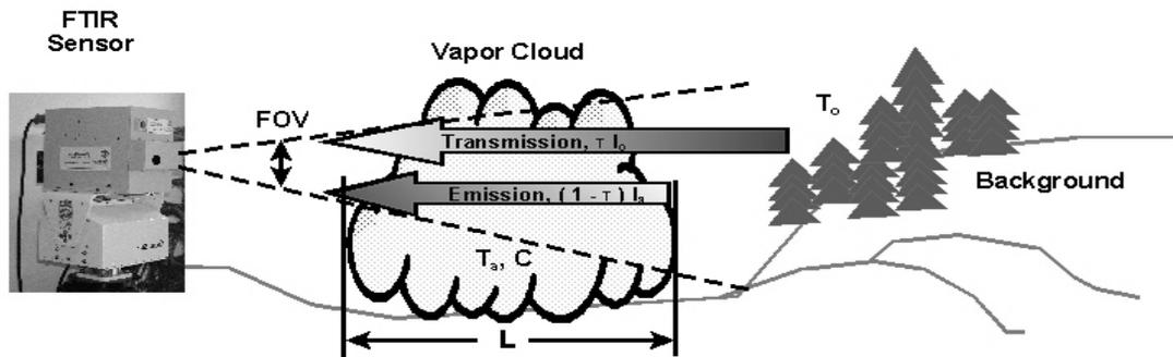
Fig. 2 – Passive FTIR sensor FGC signal model.
