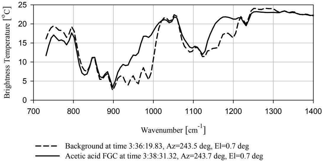
Fig. 6 – AA FGC release brightness temperature spectra.
