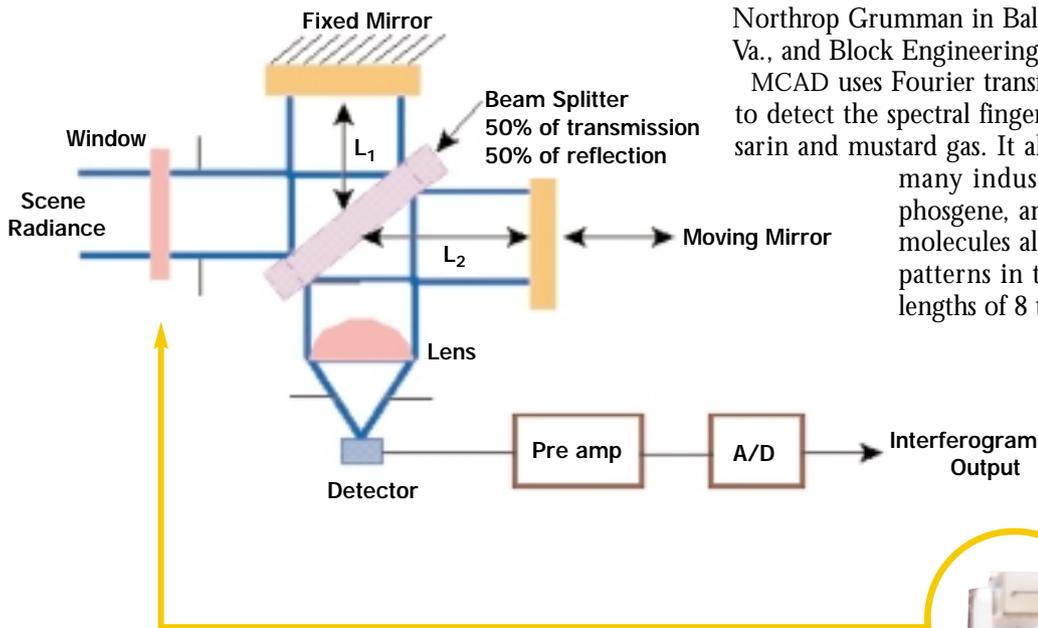
A schematic (left) of the spectrometer, compact enough to ride on an SUV.
