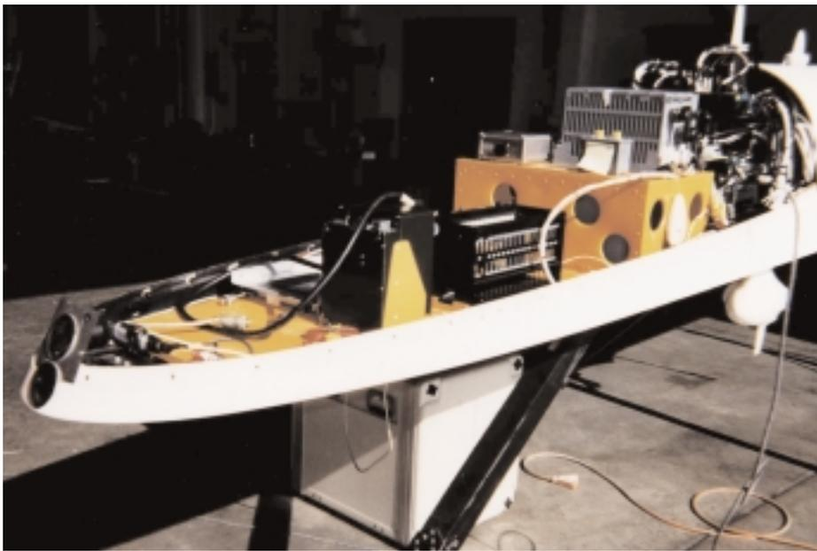
The MCAD system mounted on an unmanned aircraft. The device takes 12 infrared snapshots a second, from which chemical vapors can be identified by their spectrographic profiles.
