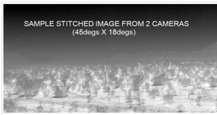
Figure 6. Sample stitched and balanced image of a mountainous desert environment using two 24deg x 18deg FOV cameras. The several degree overlap of the two cameras creates a 45deg x 18deg stitched image.
