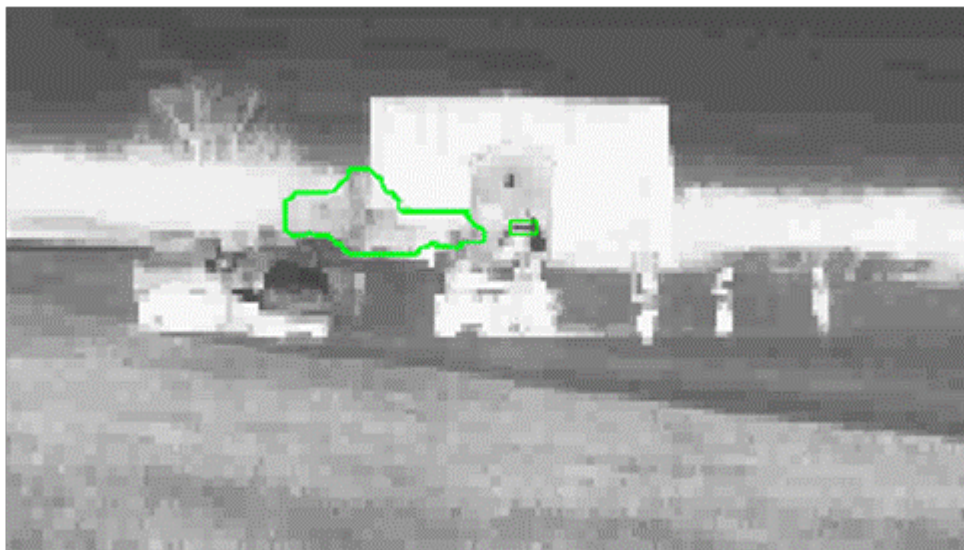
Figure 11. Tracking algorithm results for a 100-gram release of a bio simulant at a 250-meter standoff distance.
